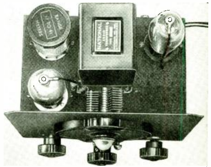
Above we have the top view, showing the arrangement of parts used in the battery operated "Economy-2."
