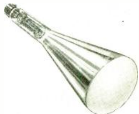
Top photo—front view of the combined "image and sound" television receiver for the Home. Center—rear view of the Loewe "home" television, and lower photo the cathode-ray or Braun tube used to reconstruct the image.
