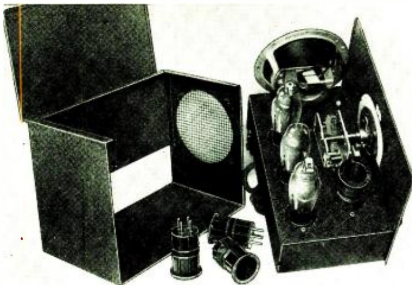
Extremely compact yet a very smooth-working set is the new Harrison "5 in 3" 3-tube S.W. receiver. It uses plug-in coils and has all the latest refinements. No. 247.
